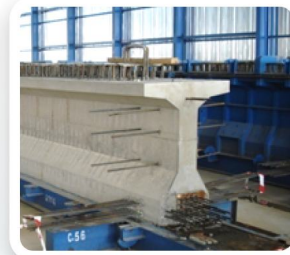
Segmental or Monolit "T" Beam
